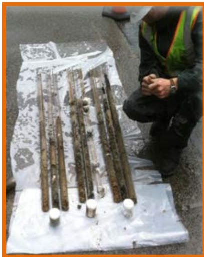
Collecting discrete samples from 40 feet of continuous soil core.
