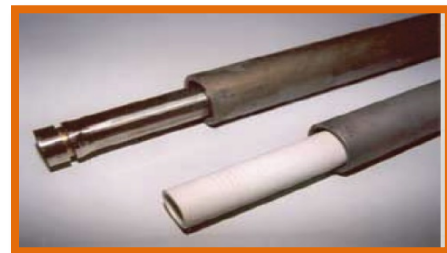
Screen Point Samplers with screen extended.
