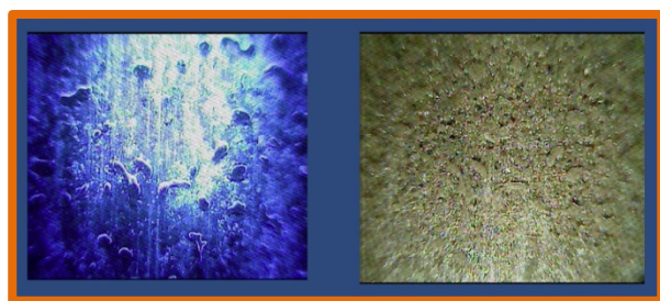
Captured image of soil fluorescence (left) and soil under visible light (right) at the same depth.
